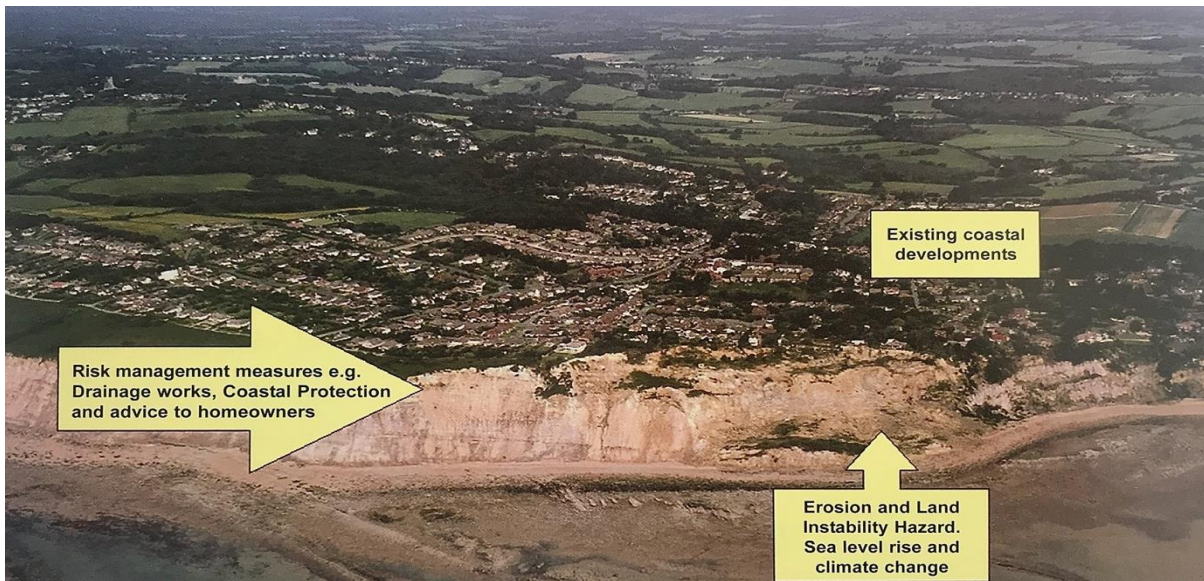
Figure 2.4: Since the late 1980s meeting the challenges of coastal risk management at Fairlight Cove has involved extensive investigations, research, physical coast protection works, drainage and updated planning policies for managing coastal land instability. Collectively, the measures provide significantly improved standards of protection for the frontage in the future.
